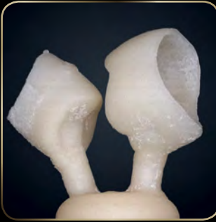
Reaction layer: Hybrid layer consisting of investment and press material
