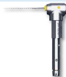
L3 Endo Head For hand NiTi files. Yellow 1:1 Transmission For root canal prep with alternating 90° rotation.
